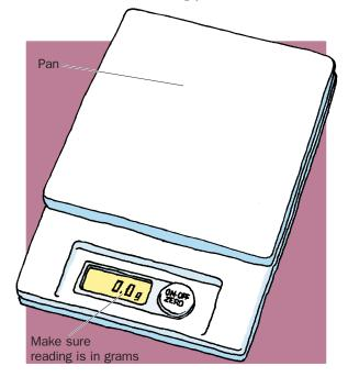
**Figure 2.1** Make sure the balance reads 0.0 g before placing an object on it.
