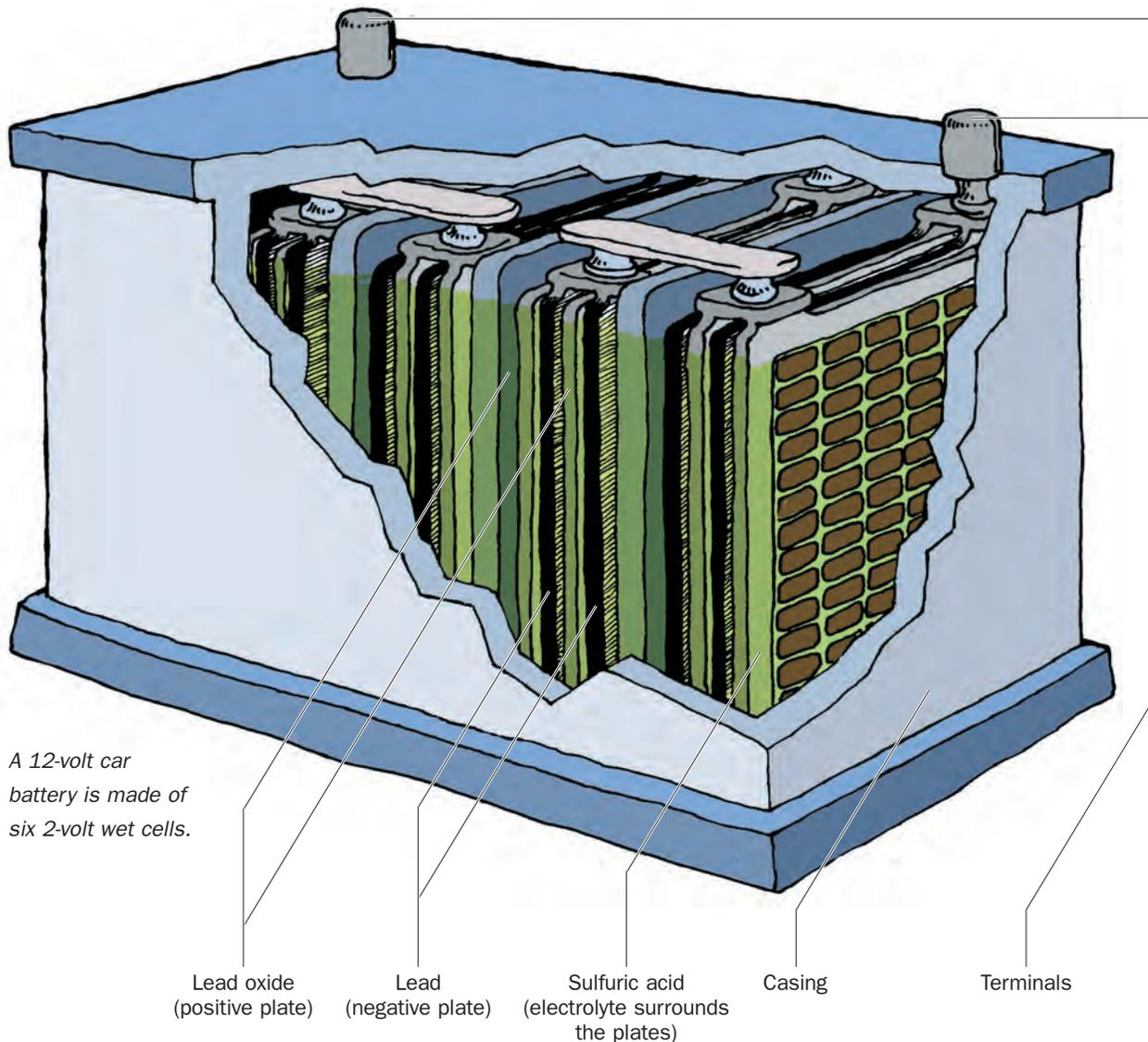
In Lesson 2, you made a battery using two metal strips, called electrodes, and a liquid, called an electrolyte. The assembly of zinc and copper strips placed in a copper sulfate solution is an example of a “wet-cell” battery. It is called “wet” because the electrodes are placed in a liquid. The copper sulfate solution was the electrolyte for your battery. The battery you made is called a cell because it is the basic building
