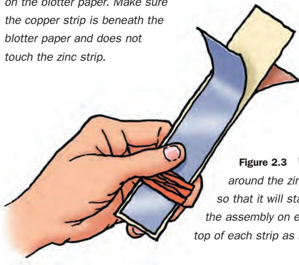
**Figure 2.3** Wrap a rubber band around the zinc-copper assembly so that it will stay together. Stand the assembly on end and bend the top of each strip as shown.
