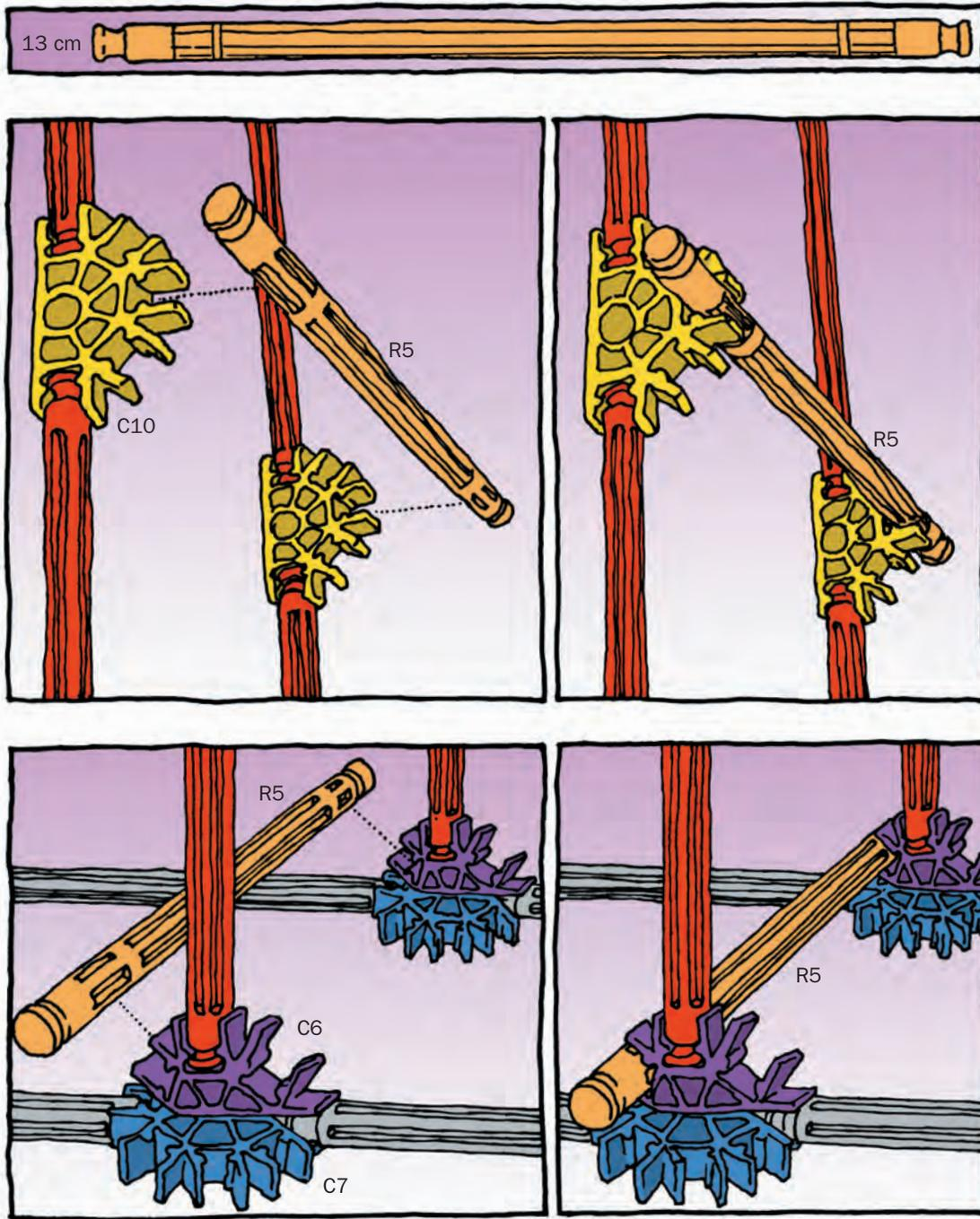
Figure 20.7 How to connect gold rods to the roller coaster
