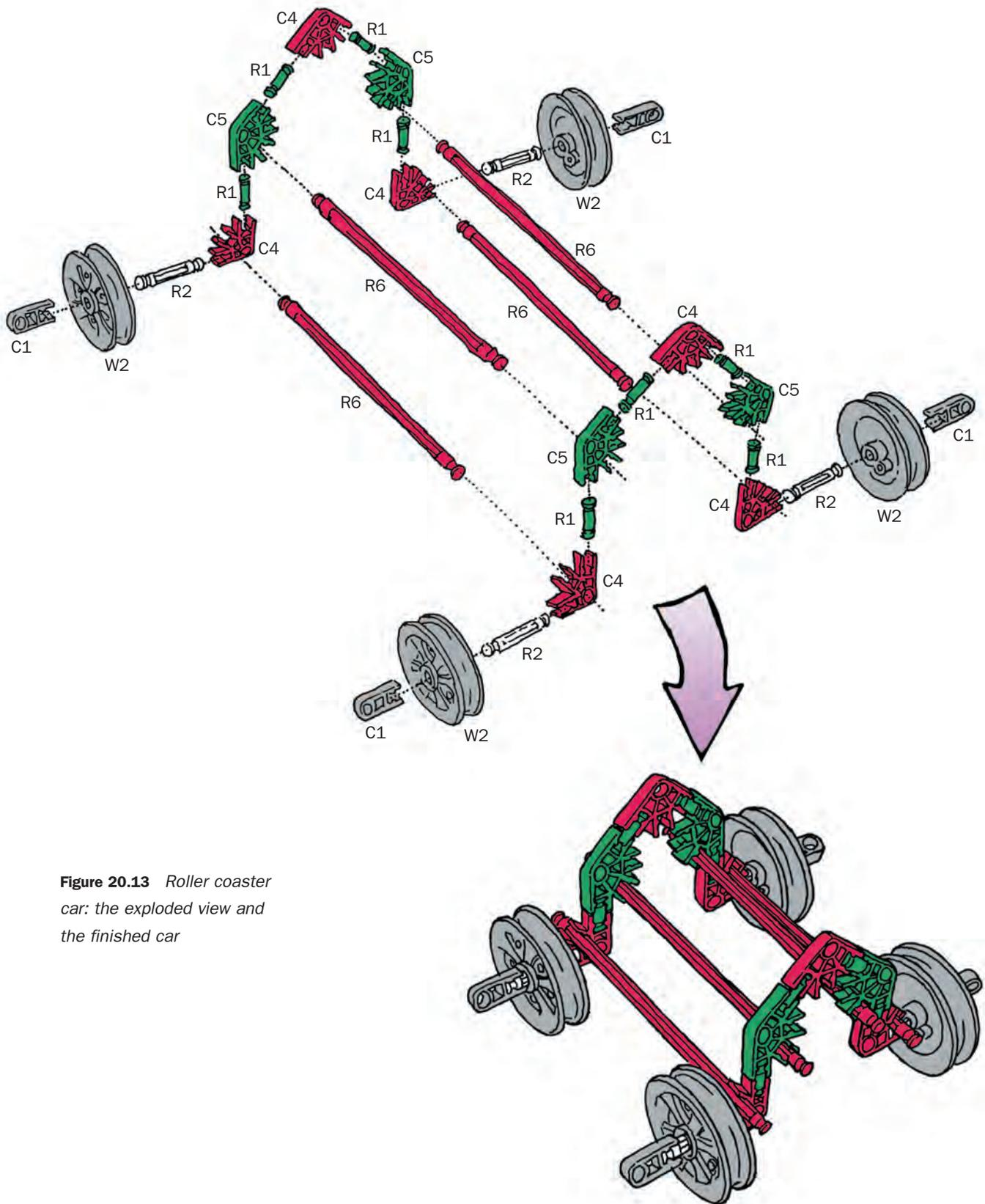
**Figure 20.13** Roller coaster car: the exploded view and the finished car
