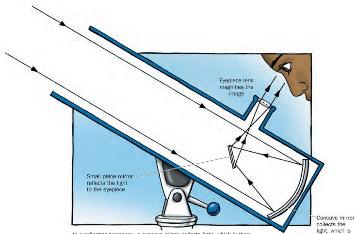
In a reflecting telescope, a concave mirror collects light, which is then directed by another mirror to the eyepiece.
