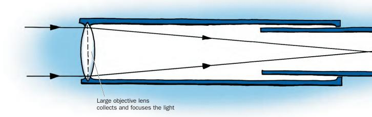
The components of a simple refracting telescope. This type of telescope is often referred to as a Keplerian telescope because it was used by the famous astronomer Johannes Kepler (1571–1630). Is the image produced by this telescope upright or inverted?
